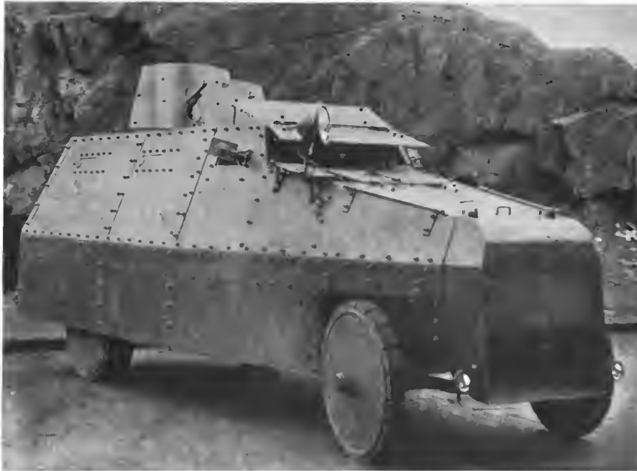
Mack AC 2-ton armored truck for N. G. N. Y. motor battery
